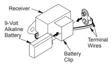
Figure 37 - Attaching Alkaline Battery to Receiver
